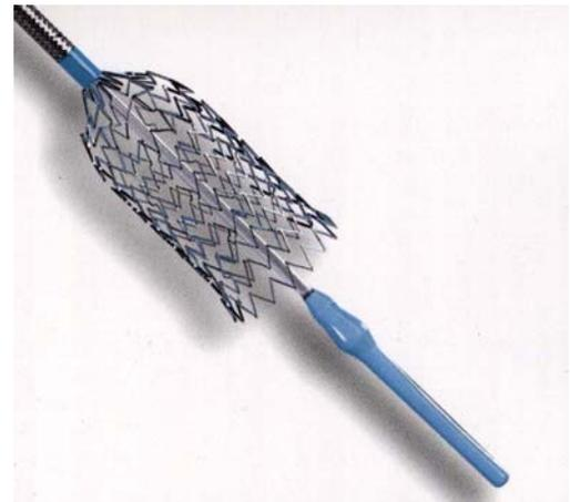
**Fig. (3).** Self expanding Nitinol stents are implanted in arteries with stenosis to reestablish blood flow. The stents are Laser cut form tube, expanded and then crimped and constrained in a delivery catheter.
