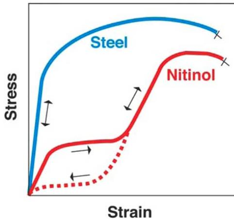
**Fig. (2).** Characteristic stress/strain curve for a Nitinol alloy wire at body temperature in comparison to steel. Deformation of more than 10% strain can be elastically recovered. This behavior is called “superelasticity”.
