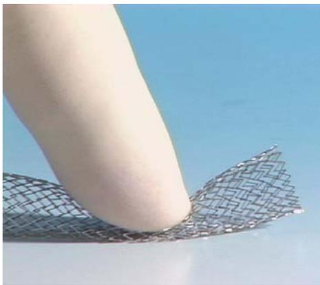
**Fig. (4).** Nitinol stents can be completely compressed (crushed) flat and will return to their original diameter when the deforming force is removed.
