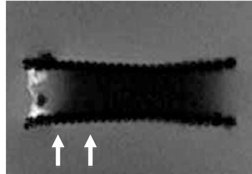
**Fig. (12).** MR visible self expanding heart valve prototype using a Bard Memotherm 22x 60 mm stent and a freshly excised porcine aortic valve [33] (see Fig. 10). The section between the white arrows contains the resonant circuit and shows the valve leaflets whereas the non-resonant section is shielding the lumen.
