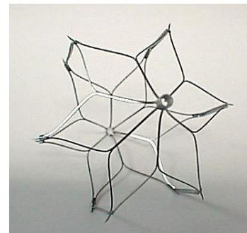
**Fig. (7).** The TrapEase vena cava filter (Cordis) consists of a monolithic structure laser cut from a Nitinol tube and expanded to its operating shape.
