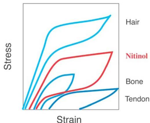
**Fig. (1).** Natural materials, like hair, tendon and bone can be elastically deformed, in some cases, up to 10% strain in a non-linear way. When the deforming stress is released, the strain is recovered at lower stresses and the loading/unloading cycle is characterized by a pronounced hysteresis. (Modified from Shabalovskaya et al. [2]).
